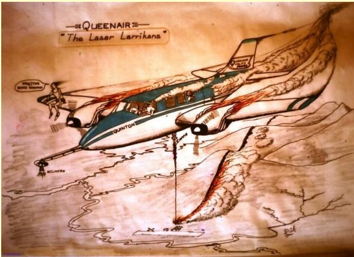
Figure 5 – believed to be a 2 Fd Svy Sqn cartoonist capturing APR Op Cenderawasih 1978 in Irian Jaya. The laser is about to cross the airfield which has a surveyed centreline vertical profile connected to the Geociever Doppler satellite station targeted with a cross allowing the sea level height of the APR crossing to be determined from the Geociever height (Source: Don Swiney)
