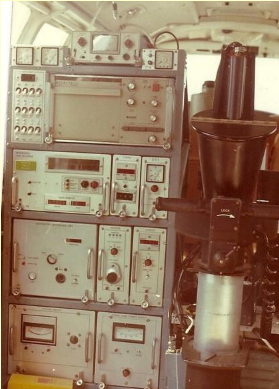
Figure 1 – WREMAPS-II installed in a Beechcraft QueenAir aircraft (VH-RUU) looking forward from the operator's seat near the aircraft door on the left. The laser, receiver and 70mm strip camera with cassette recorder are on the right with camera nearest the operator. The UV chart recorder is the large box on the right in the top rack, the digital tape recorder is the large box on the left in the next rack down next to the two laser tuners on the right and the BRU on the left in the next rack down. (Source: photo Don Swiney with component information from Ken Talbot-Smith)
