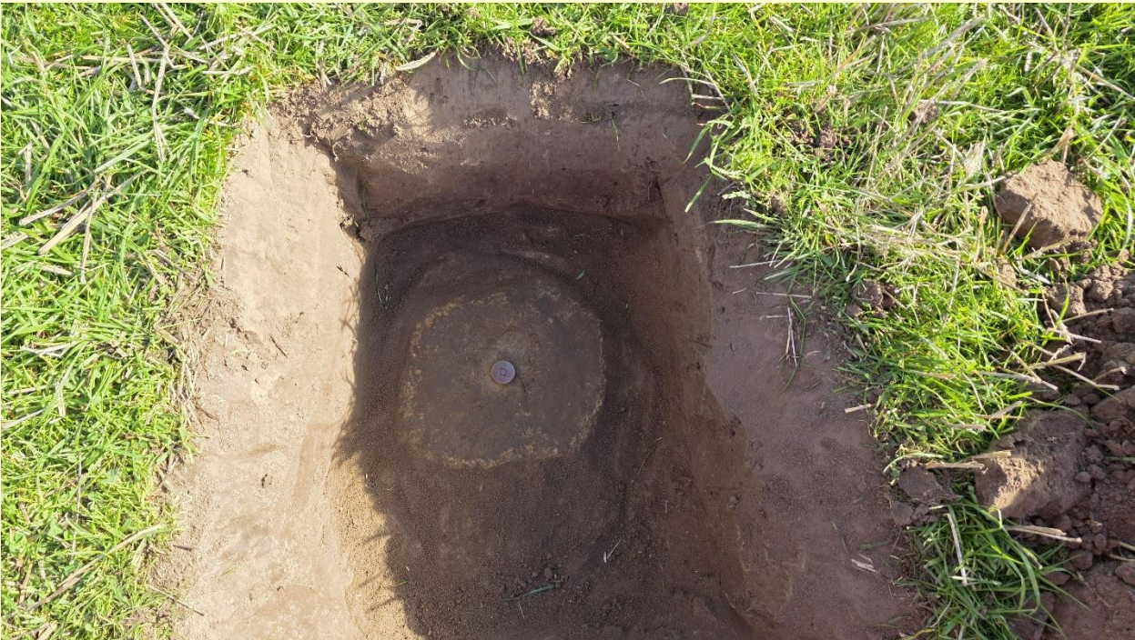
Lochmaben Astronomical Station found in 2025 - established by Aust Survey Corps in 1937. Station surface mark is 30cm below ground level as per original notes. A sub-surface mark was established about 1m below that (Photo: Adrian Fairfield)
