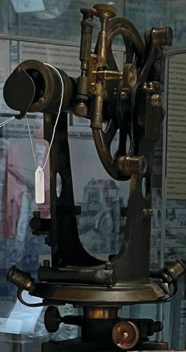
VERNIER TRANSIT AND REVERSIBLE THEODOLITE (BADIE-LONDON LR#ME 842), WITH WOODEN CARRY CASE, PLUMBBOB, SOLAR OBSERVATION FILTERS AND SPARE GRATICULE For observing horizontal and vertical angles whilst doing triangulation (surveying) in the field as part of the map making process
