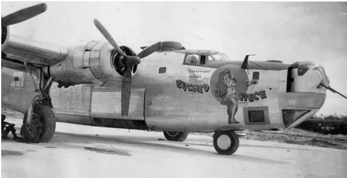
Figure 13. A F-7A B-24 Liberator photographic plane of 20 th Combat Mapping Squadron, 6 th Photographic Group, 5 th Air Force in SWPA 1944-1945. This F-7A had three cameras in the nose (K-17 trimetrogon and K-18) and three cameras in the rear bomb bay. Long-range fuel tanks were installed in the forward bomb bay. The F-7B with six cameras in the bomb bay did replace the F-7A in this squadron in late-1944. The small graphics below the cockpit window are 'air cameras' depicting the number of mapping missions by the aircraft. This F-7A went on to fly 32 missions over New Guinea, Dutch New Guinea and Netherlands East Indies.
