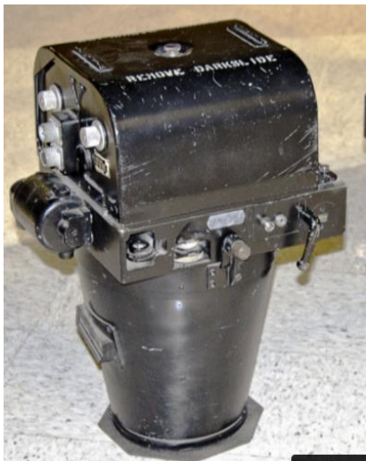
Figure 5 – Fairchild K-17 aerial camera with probably a 12-inch lens cone
