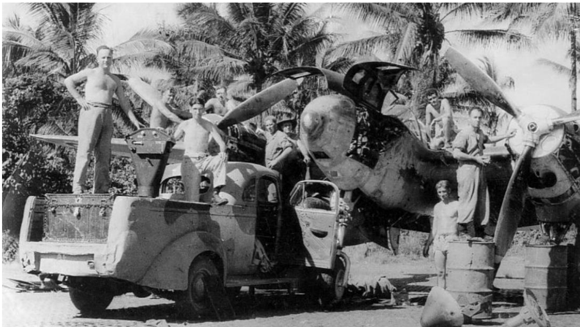
Figure 9 - An 8 th Photo Sqn F-4 P-38 Lightning – a K-18 24-inch (9x18 inch film) reconnaissance camera is standing in the back of the ute (Lockheed files)
