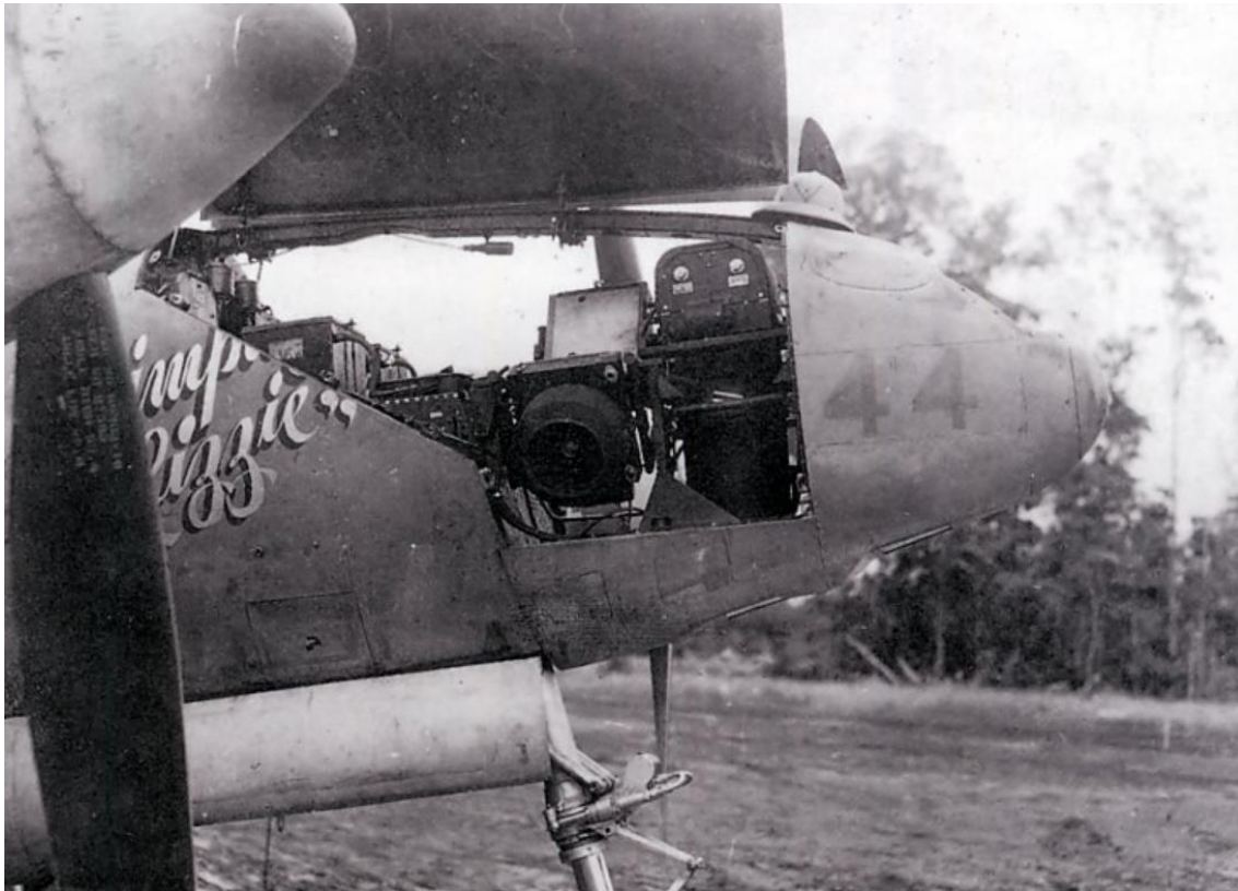
Figure 8 - An 8 th Photo Sqn F-4 P-38 Lightning Limping Lizzie – the nose camera bay showing the starboard K-17 6-inch high oblique (60 degrees off vertical) camera part of the trimetrogon system just in front of the line of the nose wheel and what appears to be a K-17 24-inch vertical camera forward of that. This was one of two F-4 Lightnings loaned to 75SQN RAAF at Milne Bay, August-December 1943 (Lockheed files)
