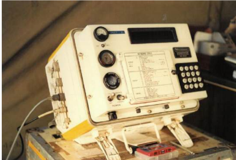
Figure 7. Op ARIGHT 85 Cape York (Det 1 Fd Svy Sqn) MX-1502, the data was recorded on the red cassette tape – the tape drive is behind the water tight cover with the Keyboard Code index (Photo: Mick McConnell)
