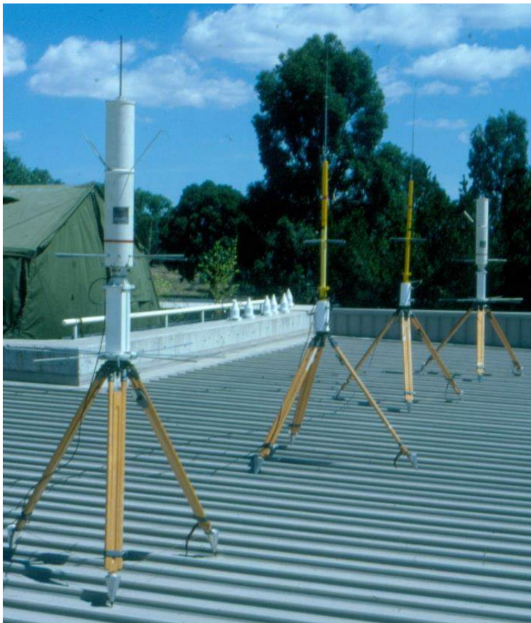
Figure 8. Two MX-1502 antennas between two AN/PRR-14 Geociever antennas at School of Military Survey in Feb 1987 for acceptance trials of TI4100 GPS geodetic receivers. The MX-1502 were observing ‘translocation’ and the AN/PRR-14 were observing simultaneous ‘point positions’. Six TI4100 GPS antennas are on the concrete in the background awaiting their turn on the tripods. (Photo: author)
