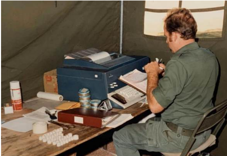
Figure 46. Op NEURATION 1983. A RA Sigs Signaler copying AN/PRR-14 Geoceiver punch paper tapes on the messaging Telex machine. Two HP9863A tape readers to convert paper tape to magnetic cassette tape on HP9815A went unserviceable from dust ingress. The small white items on the table bottom left are the Geoceiver rolled paper tapes being one for each Transit satellite pass. The round tins next to the Telex were used to store the tapes in the field. They were 'tobacco' tins with a screw-tight seal. The supply battalion questioned why we were buying 'tobacco' tins (empty). They were more mystified being told they were for data recorded from observations of satellites. (Photo: Mark Heinrich)
