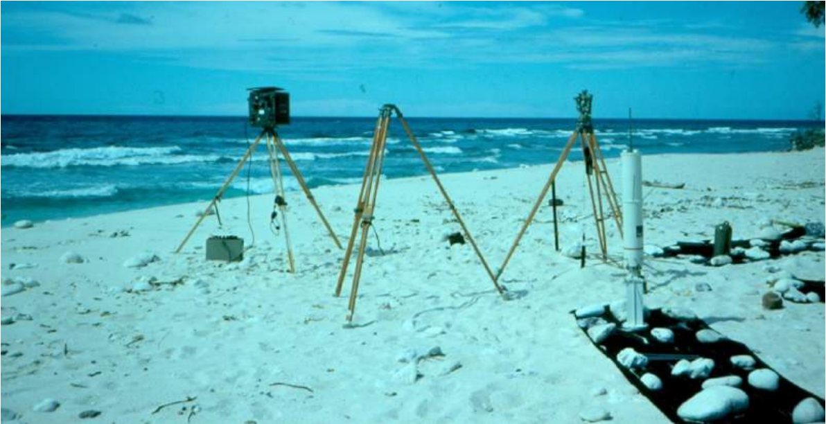
Figure 13. Op CENDERAWASIH 1976 Irian Jaya, Indonesia - Island surveys were often a combination of Geociever at one point to establish an absolute 'point position' then a reciprocal sun azimuth (Wild T2 on the tripod above the ground mark) and Tellurometer MRA301 (on the left on a 90 deg offset eccentric) distance to establish another point at the other end of the island for azimuth and scale. The Geociever antenna is standing on a black cloth bunting panel used here for station identification photography (Wild RC10 mounted in an AAAvn Pilatus Porter) against a highly reflective white sand background. The station identification photography was flown while the Geociever team was on site to make sure the black panels were visible. This was one of the stations when the mapping photography (2 Sqn RAAF Canberra, Wild RC10, 40,000ft) was also flown when the Geociever team was on station. (Photo: author)
