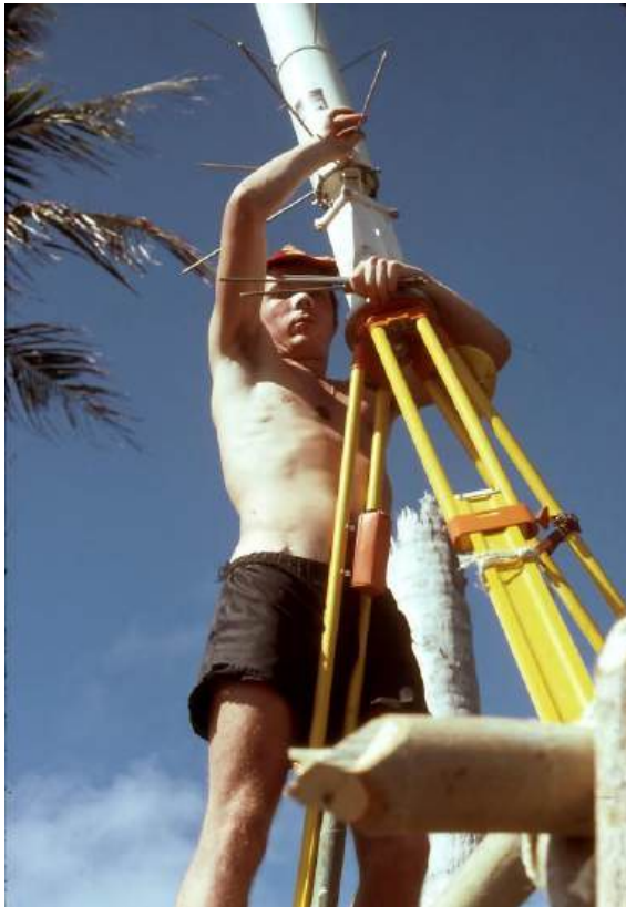
Figure 29. Op SPEARLINE 1980 – Sapper Andy Capp 80 on a log tower, screwing in the Geociever antenna ground-plane rods (Photo: Brian Partridge)
