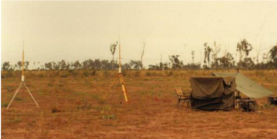
Figure 49. Op ARIGHT 85. Det 1 Fd Svy Sqn MX-1502 believed to being tested at Weipa Airport Main Base. The antenna and tripod on the left is a loan MX-1502 from QLD Lands Dept (Photo: Mick McConnell)
