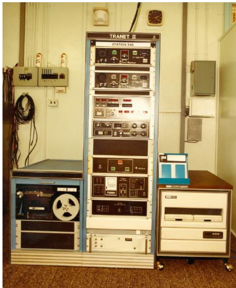
Figure 1c. TRANET II Station 545 Smithfield SA – next to the GPS receiver equipment (p17) not in this photograph. Note the first generation 8-inch floppy disc removable media on the floppy drive cabinet. (Photo: the author 1983)
