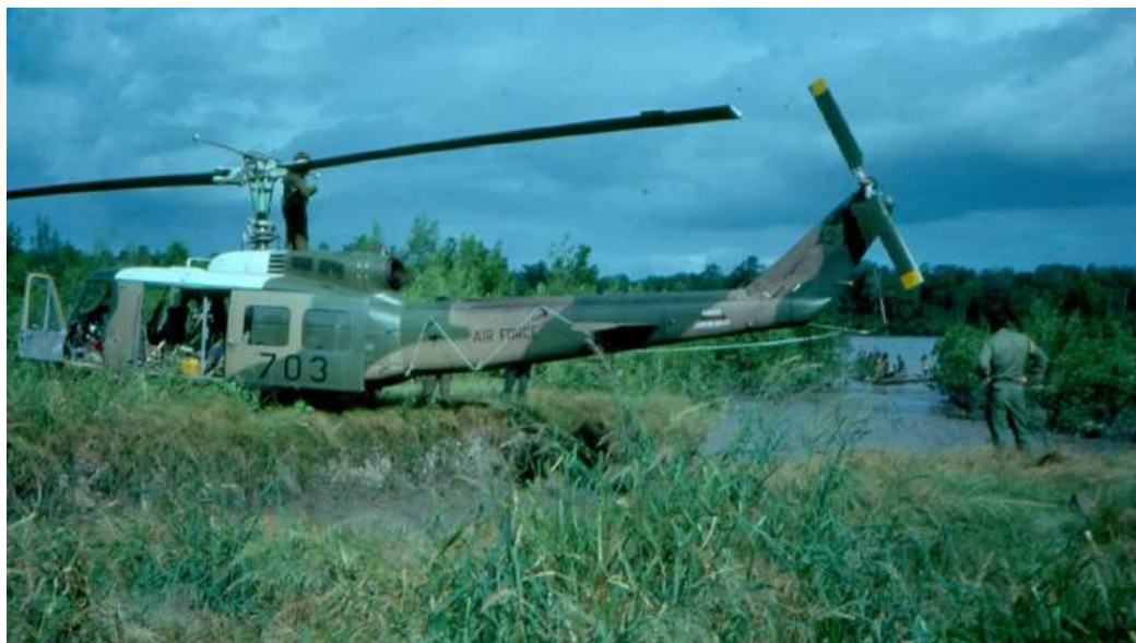
Figure 22. Op CENDERAWASIH 1977 Irian Jaya, Indonesia – the Geociever reconnaissance team testing an Iroquois landing zone making sure the aircraft didn't sink in the surface mud at a chosen Geociever site near AGATS on the south-east coast. Sapper Jamie Lyle 67 , near the Iroquois tail rotor, is making contact with locals in the canoes coming to see what was going on. Jamie was a great asset on reconnaissance, having attended with distinction the short Indonesian language course at RAAF School of Languages at RAAF Base Point Cook. (Photo: author)
