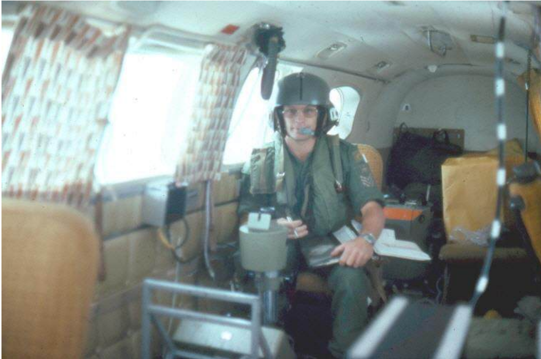
Figure 30. Op SPEARLINE 1980 – Staff Sergeant Brian Partridge in the charter Queen Air at the Wild RC10 air camera NF2 navigation sight. Brian achieved the first mapping photography of Malaita Island a feat much appreciated by the Surveyor-General Solomon Islands who presented Brian with a carton of beer. (Photo and story: Brian Partridge)
