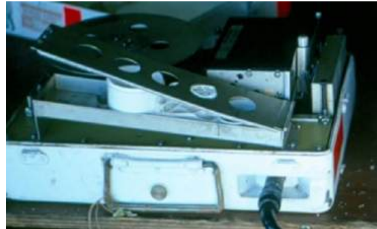
Figure 4a. AN/PRR-14 Geoceiver – punch paper tape recorder. The paper tape for each pass spooled into the tray with holes in the top. After the pass, the tape was annotated with station and pass information, rolled up and stored in a circular cigarette tobacco tin with a screw seal lid. The daily ‘mode’ and ‘alternate data’ checks were also recorded on the punch paper tape then deciphered manually (Photo: author).
