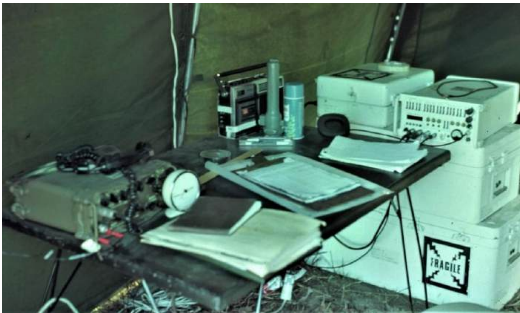
Figure 4. Op CENDERAWASIH 76 AN/PRR-14 Geoceiver – receiver on the right, punch paper tape recorder (lid closed) next to it, both on the white watertight transit boxes. The bottom transit box is for the antenna and the other is for the receiver. The HF radio AN/PRC-F1 is on the left. The alarm clock was set to UTC which was the satellite pass prediction time. The satellite prediction computer printout is in the folder in the foreground. The personal short-wave radio kept the team in touch with world news and music. (Photo: Gary Hunter)
