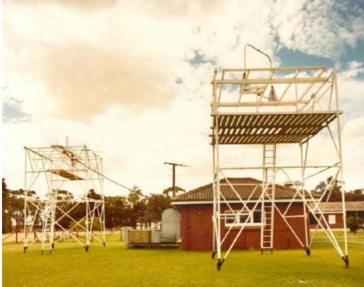
Figure 1b. TRANET Smithfield SA – west antennae platform (left) above a RA Svy plaque and east antennae platform (right) above a John Hopkins University plaque. The tracking and recording equipment is in the red brick building. (Photo: the author 1983)
