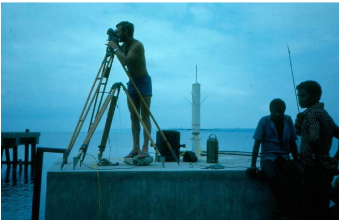
Figure 16. Sapper Wally Chilcott 63 (2 Fd Svy Sqn – Topographic Surveyor) observing (Wild T2 theodolite) the vertical angle to a tide gauge. This was an observed vertical survey connection between sea-level (the geoid from the tide gauge) and the spheroid (from the Geociever). (Photo: author)
