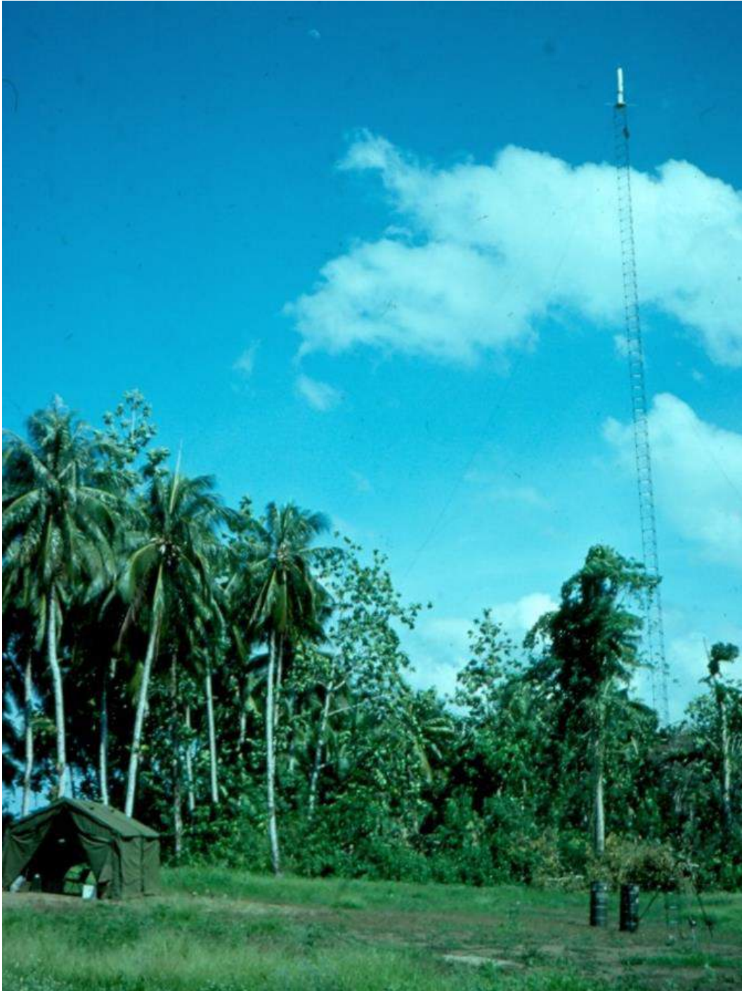
Figure 6. AN/PRR-14 Geociever antenna atop a 75 foot Canadian Astromast. This tower is intentionally leaning to place the station ground mark plumb under the antenna using a Wild T2 theodolite. The two storage/transport drums and the winch tripod are near the base of the tower. The antenna/pre-amplifier is connected by a 100 foot coaxial cable to the receiver in the tent. (Photo: author)
