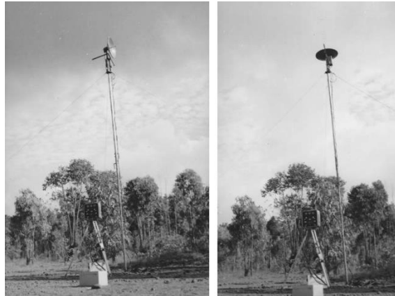
The AERODIST MRC2 Remote (on the tripod) antenna could be mounted on a 20 foot pole tower. The antenna direction was controlled by wires/ropes to the two arms under the dish at right angles. The antenna elevation could be changed to the vertical for aircraft height checks (right photo). (Photos: 4 Fd Svy Sqn)
