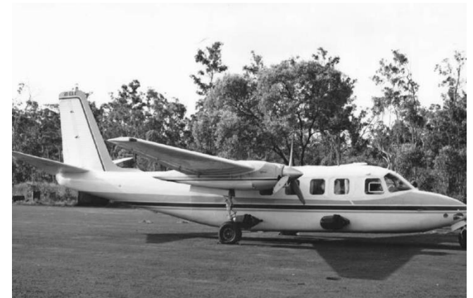
Aero Commander VH-EXX at Gove NT. AERODIST antenna pods in the rotated raised position are on the aircraft fuselage. (Photo: 4 Fd Svy Sqn)
