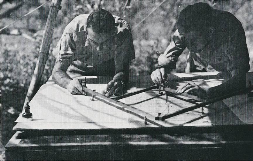
Figure 9: Drawing a map sheet using a pantograph to change scale, Adelaide River 1942
